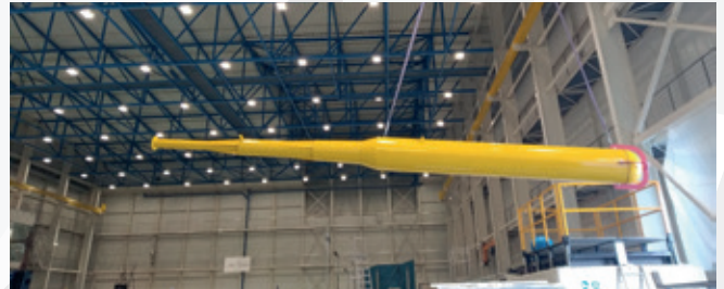
Picture of the spar prototype tested in Environmental Hydraulics Institute of Cantabria's basin. Source: IHCantabria.
