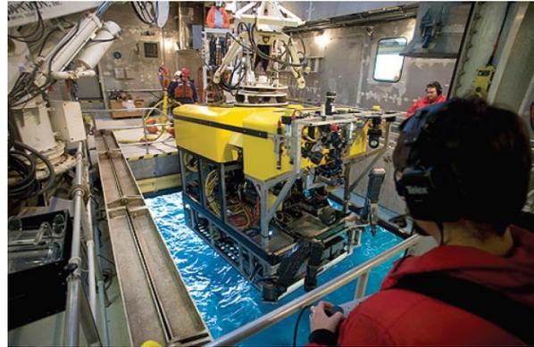
Figure 22: ROV being launched through moonpool; [source: [50]].
