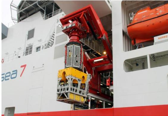
Figure 21: A-Frame preparing for launch, [source: [62]].
