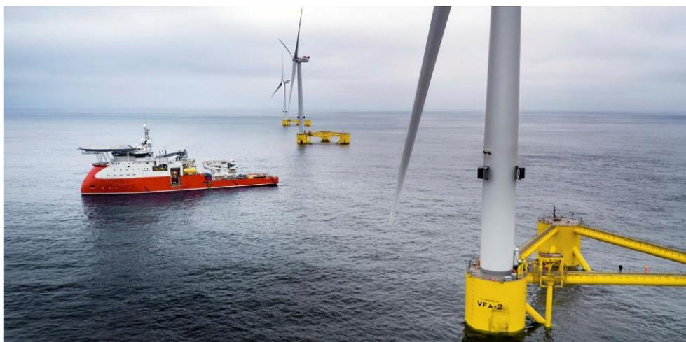
Figure 33: WindFloat Atlantic with additional spar attached to the floating substructure, [source: [100]].
