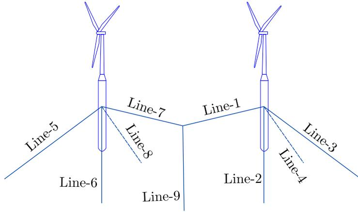
Figure 18: Shared mooring line design with 2 turbines in Morro Bay site
