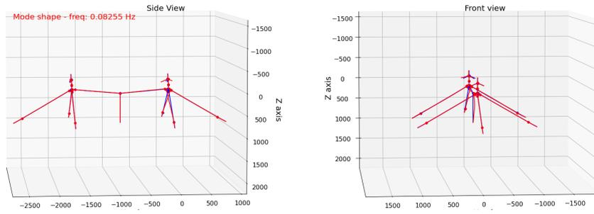
Figure 31: The first yaw mode shape of Design-3
