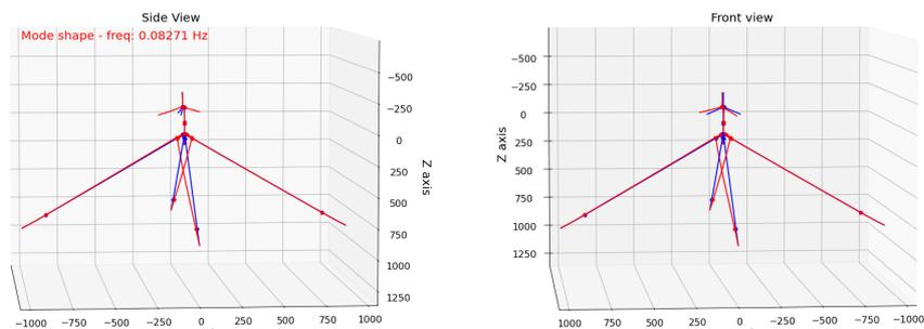
Figure 29: The first yaw mode shape of the single turbine design
