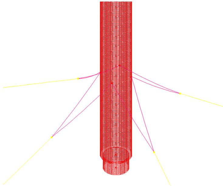
Figure 41: Bridle Chains Connecting to Spar
