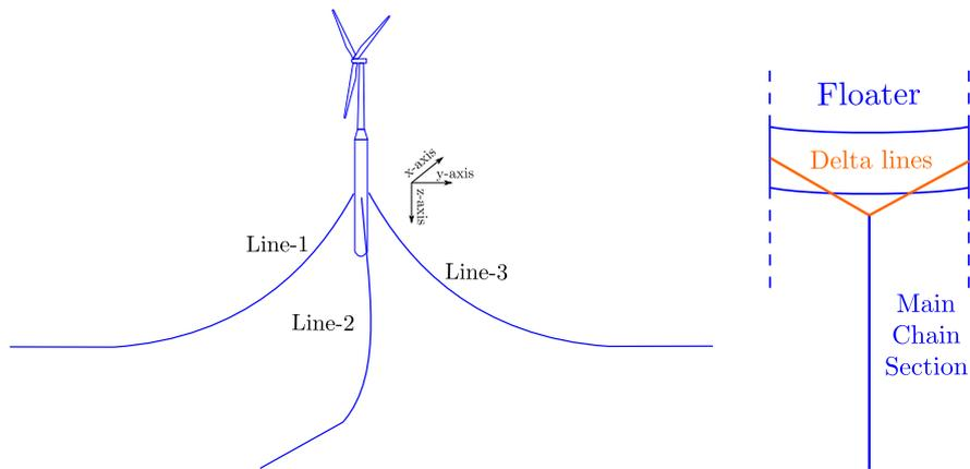
Figure 8: Single turbine design in Grand Canaria site and mooring line segments
