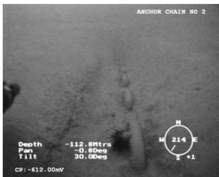
(c) Mooring chain on seabed showing no visible twist [Source: [17]].
