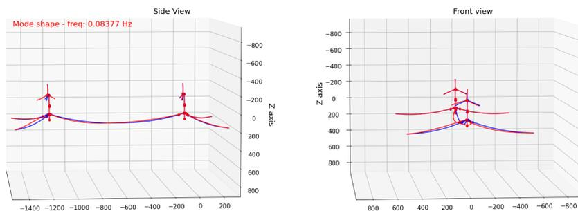
Figure 15: Design-1 mode shape at 0.0838 Hz
