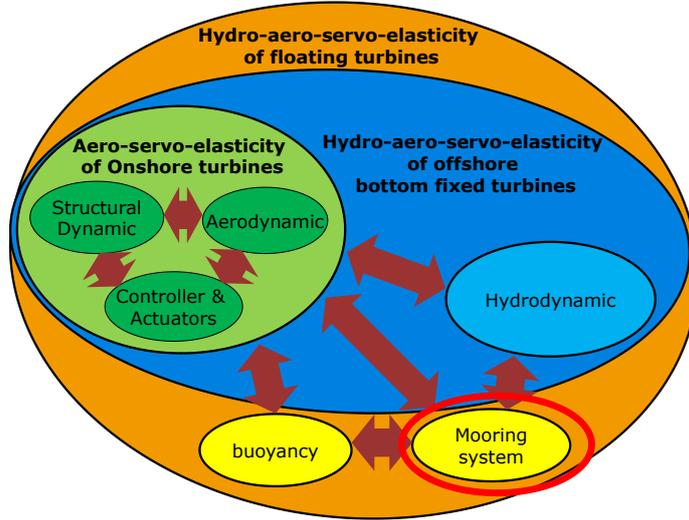
Figure 6: Wind turbine load computation sub-modules for different turbine configurations
