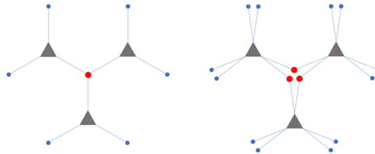
Figure 5: Illustration of exemplary configurations for shared anchors (red dots) [Source: Ramboll].
