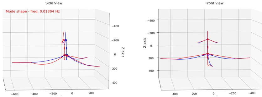
Figure 11: Single turbine case first mode shape
