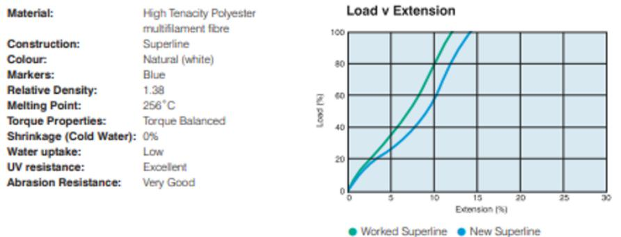
Figure 39: Polyester Superline Load vs Extension Curves [7]
