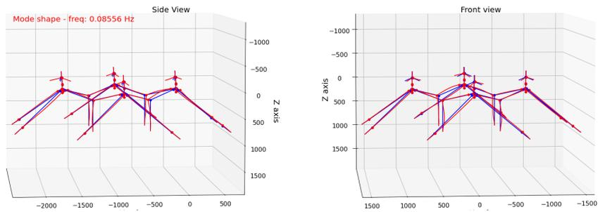
Figure 37: Mode shape of the system at 0.0856 Hz
