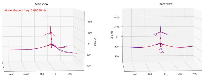
Figure 14: Single turbine mode shape at 0.0906 Hz
