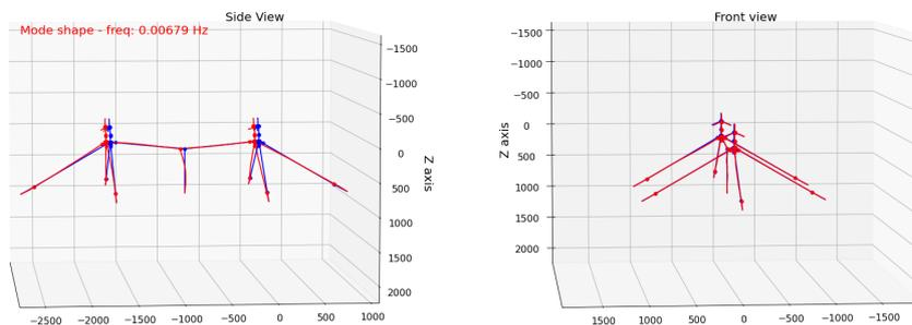
Figure 23: Symmetric surge mode shape for Design-1 which has zero buoyancy force at the intersection
