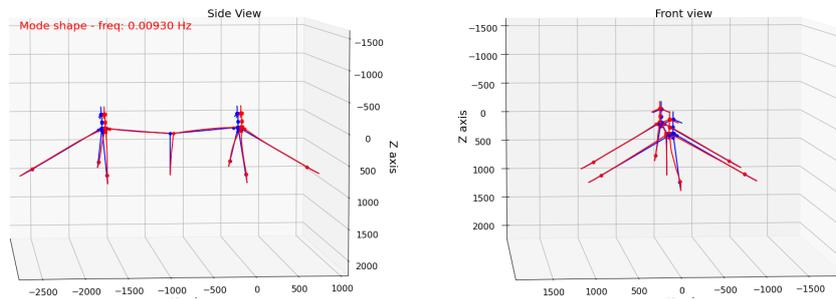
Figure 28: The first mode shape of Design-5
