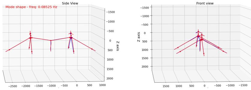
Figure 32: The first yaw mode shape of Design-5
