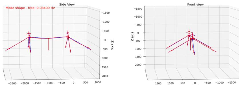
Figure 30: The first yaw mode shape of Design-1
