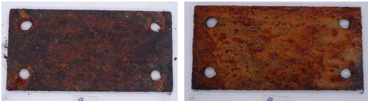
Figure 3-12. Plate # 8: Bare steel at Tidal area. Face A (left) and Face B (right)
