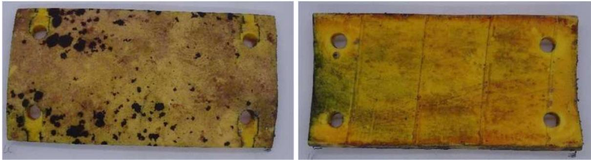
Figure 3-11. Plate # 5CC: Cable coating at Tidal area. Face A (left) and Face B (right)
