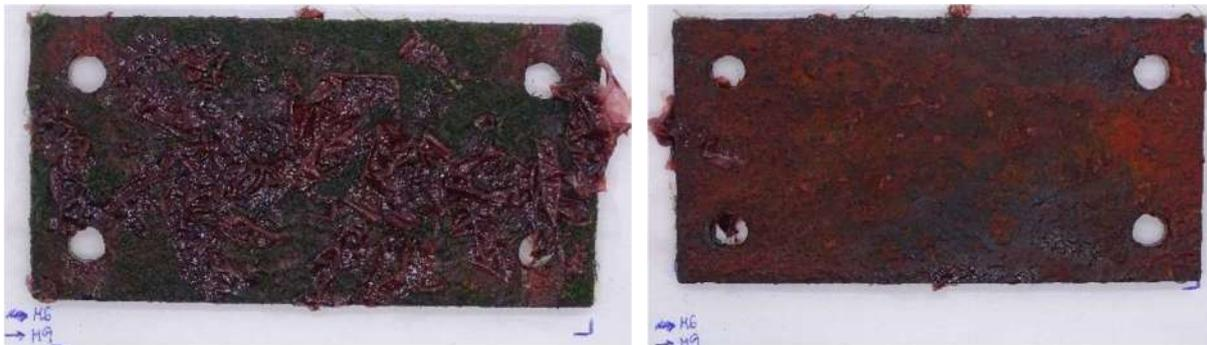
Figure 3-10. Plate # 4: Bare steel at Tidal area. Face A (left) and Face B (right)
