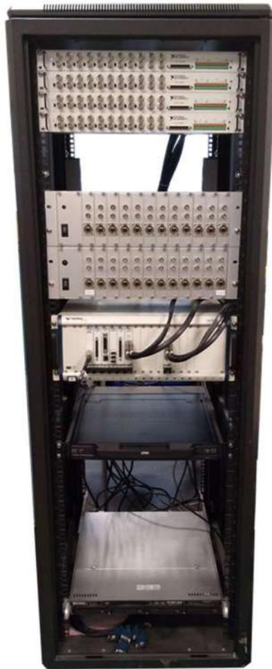
Figure 4-35. Acquisition system cabinet based on NI PXI chassis
