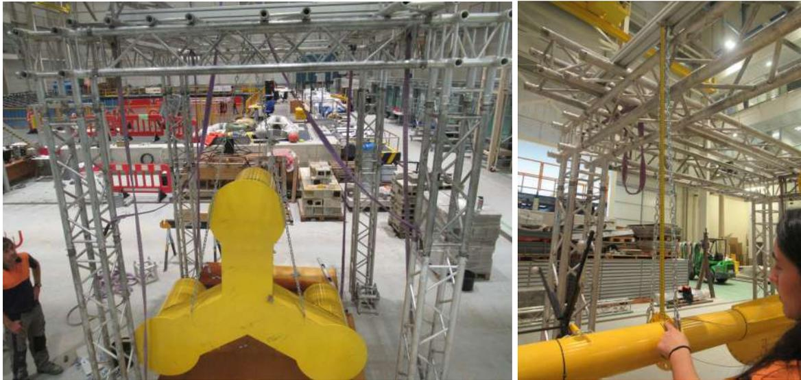
**Figure 4-24. Izz Inertia test (left) and detail of hanging (right)**
