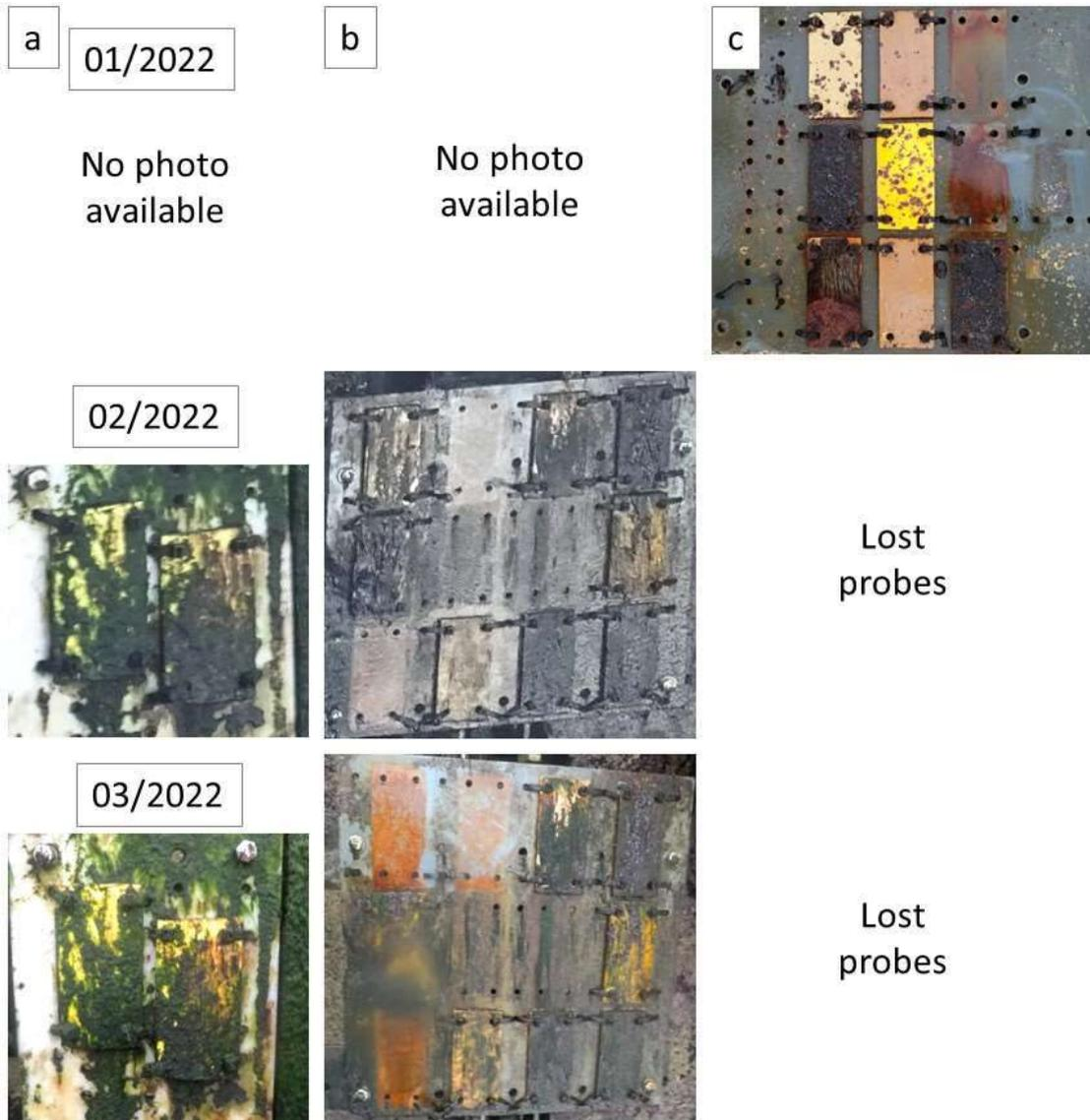
Figure 3-5. State of the plates between January 2021 and March 2022. Column a: Splash level; Column b: Tidal level; Column c: Submerged level.
