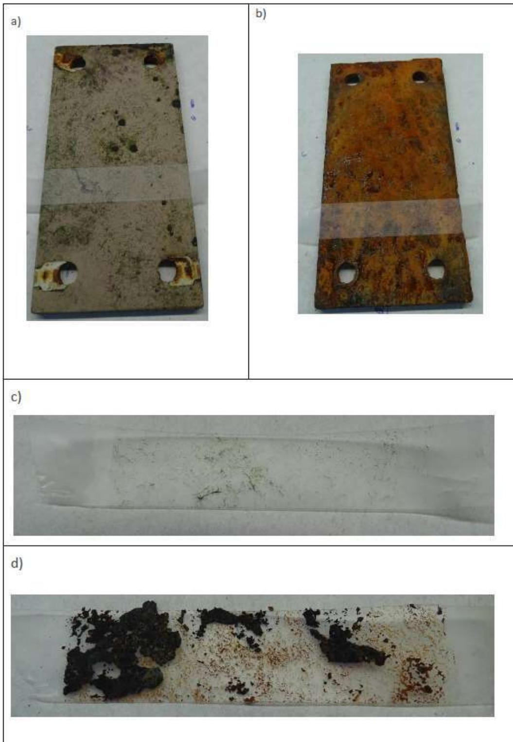
**Figure 3-33. Plate # 6: Face A (top left), Face B (top right), Chalking adhered to the tape in Face A (centre) and Chalking adhered to the tape in Face B (bottom)**
