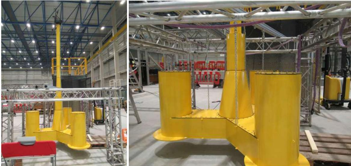
Figure 4-21. Weight, CoGx and CoGy position test (left) and detail of hanging (right)
