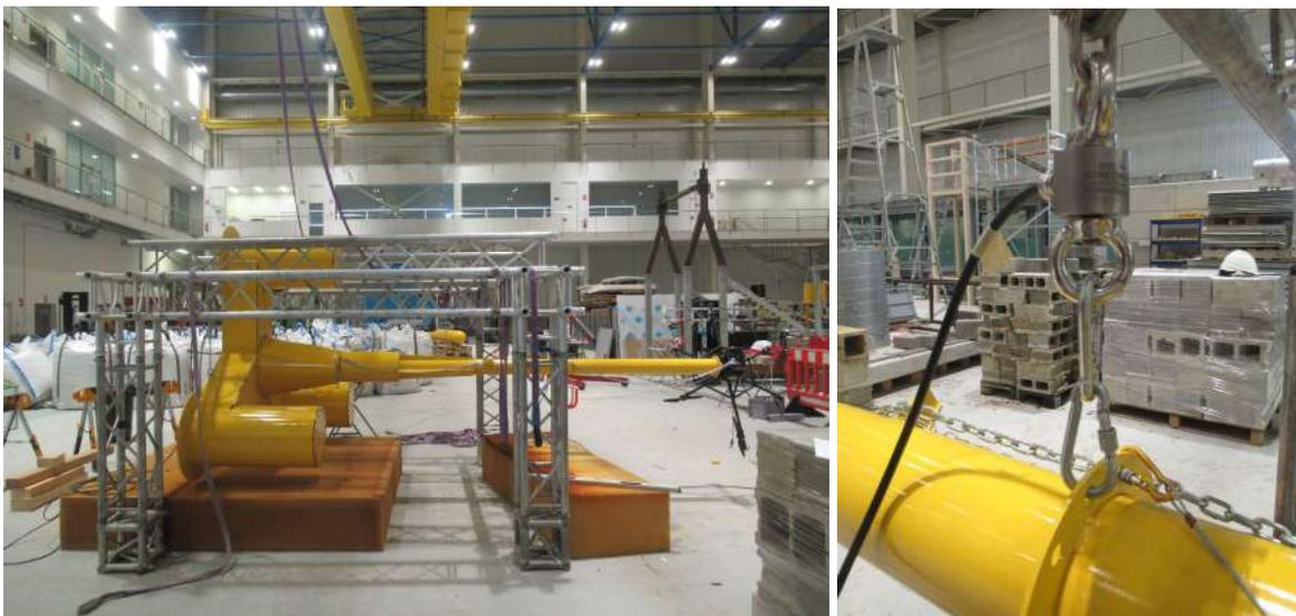
Figure 4-22. Weight and CoGz position test (left) and detail of hanging (right)
