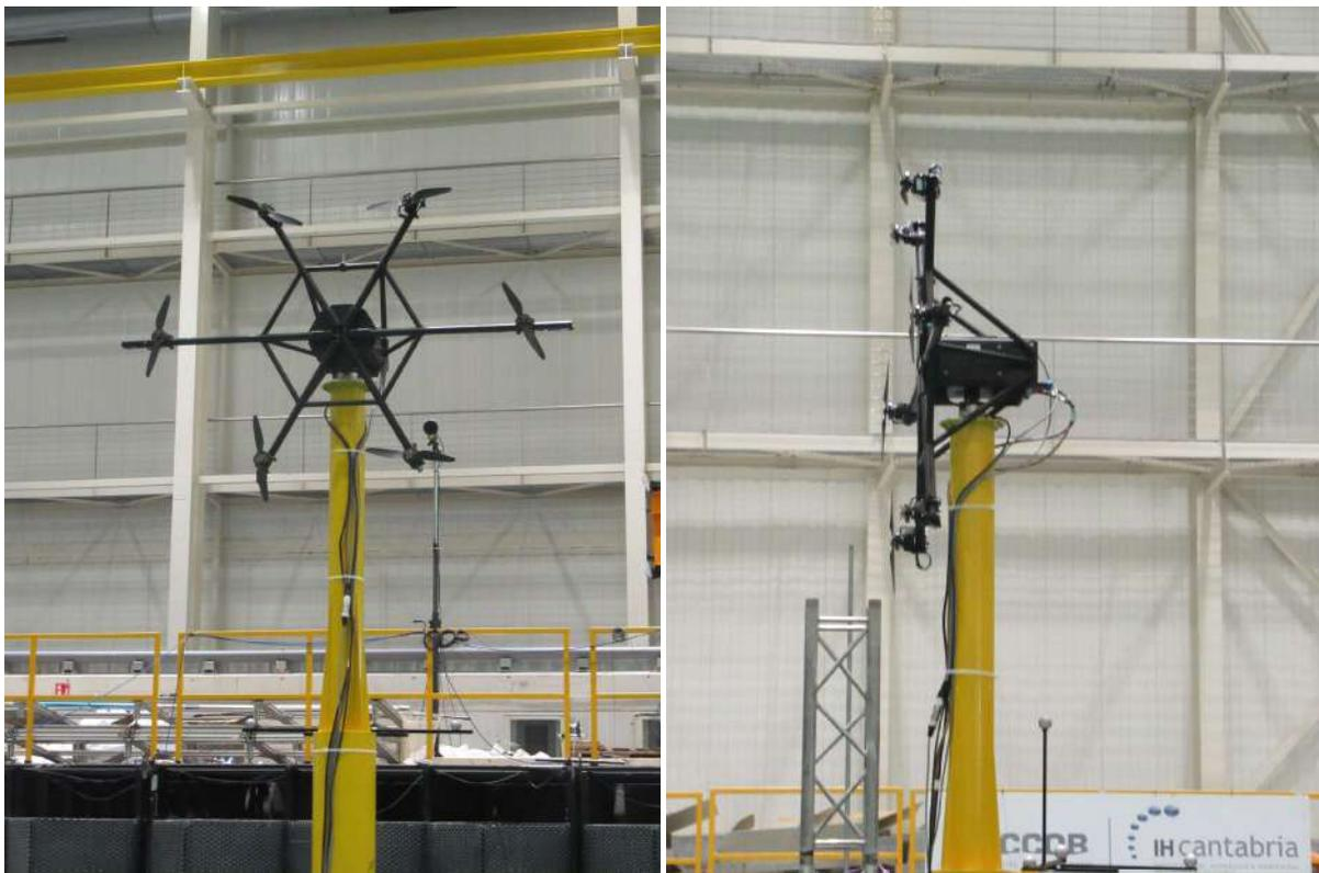
Figure 4-17. FIHAC Multi-fan mounted on the top of the mockup
