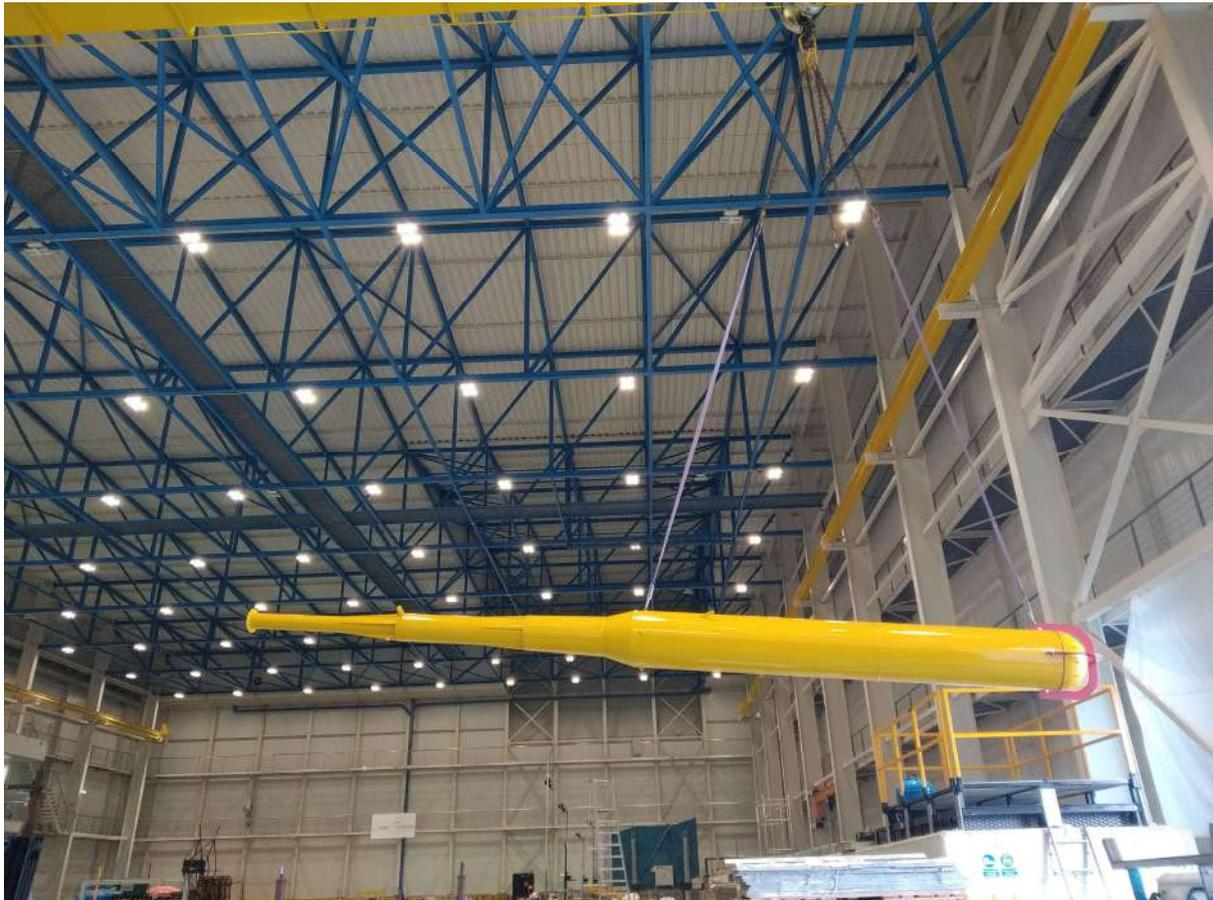
**Figure 4-5. WINDCRETE manufactured mockup being hung by the lugs at FIHAC facility**
