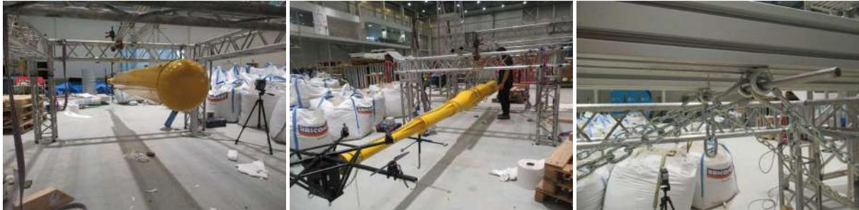
Figure 4-7.  $I_{xx}$  Inertia test (left)  $I_{yy}$  Inertia test (centre) and detail of hanging (right)
