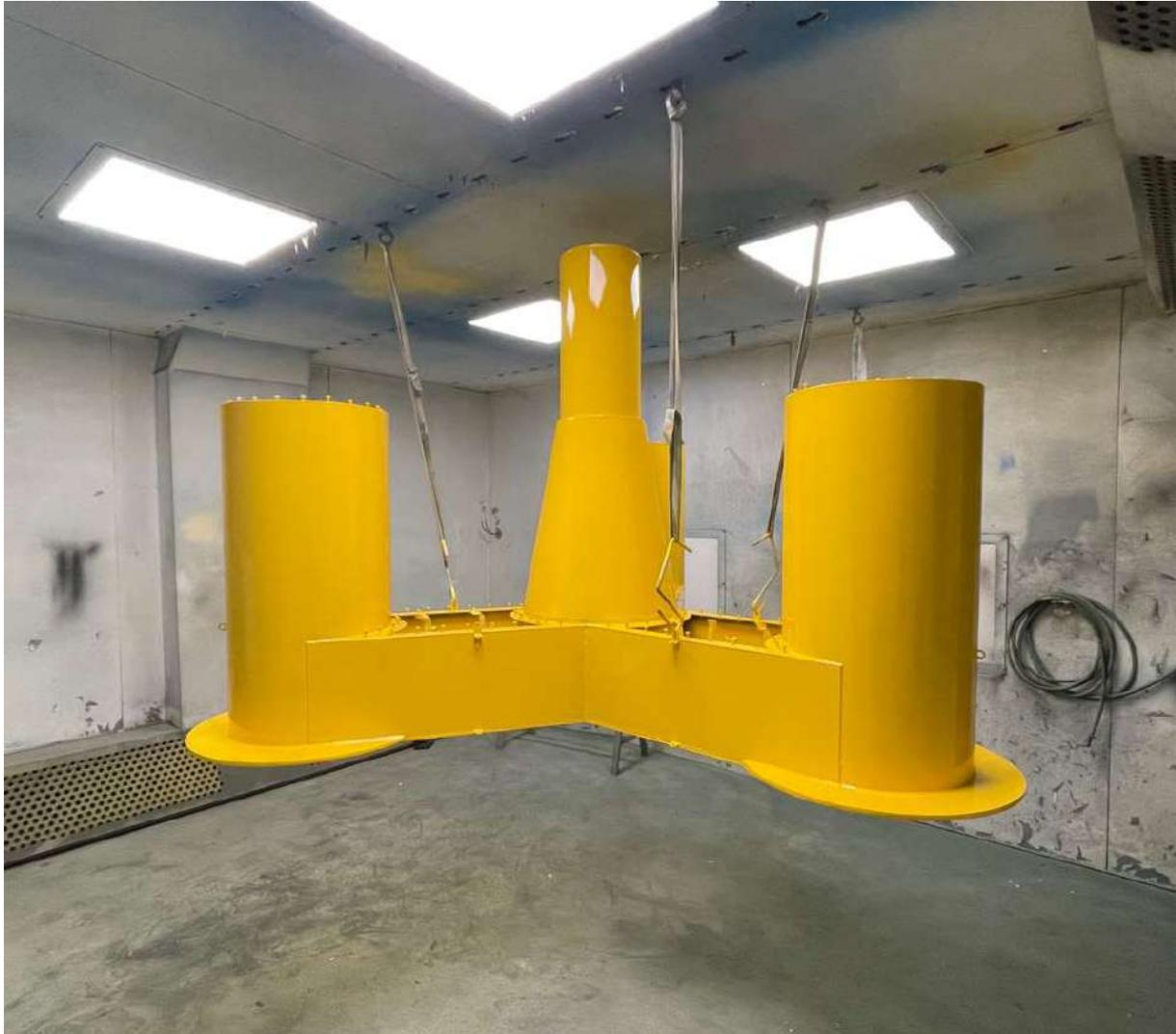
**Figure 4-20. ACTIVEFLOAT substructure mock-up hung by the lugs after being painted in yellow**
