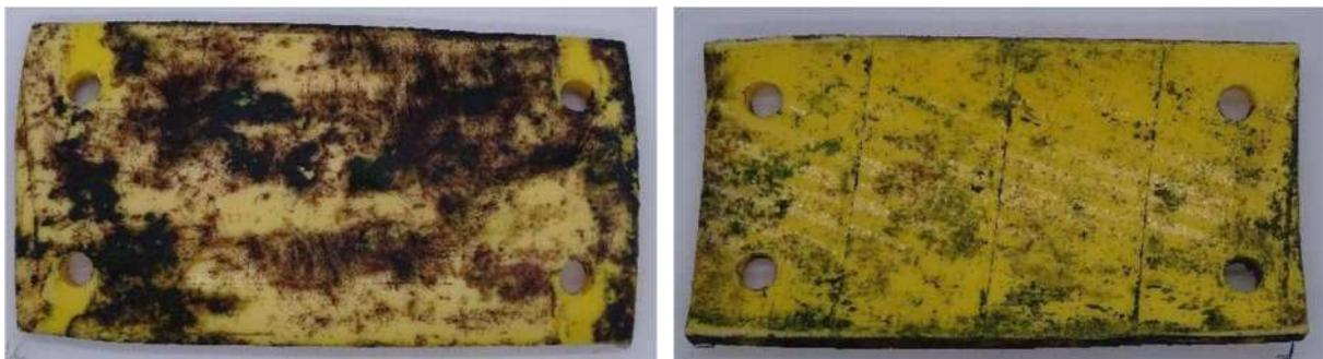
Figure 3-10. Plate # 4CC: Cable coating at Splash zone. Face A (left) and Face B (right)
