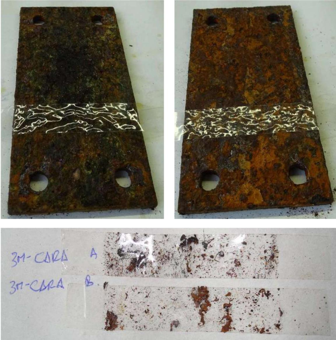
Figure 3-36. Plate # 4: Face A (top left), Face B (top right) and Chalking adhered to the tapes (bottom)
