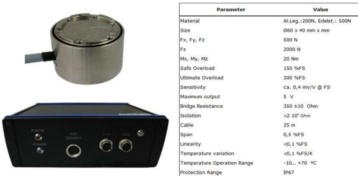
Figure 4-40. K6D40 multi-axis force transducer and amplifier (left) technical specifications (right)
