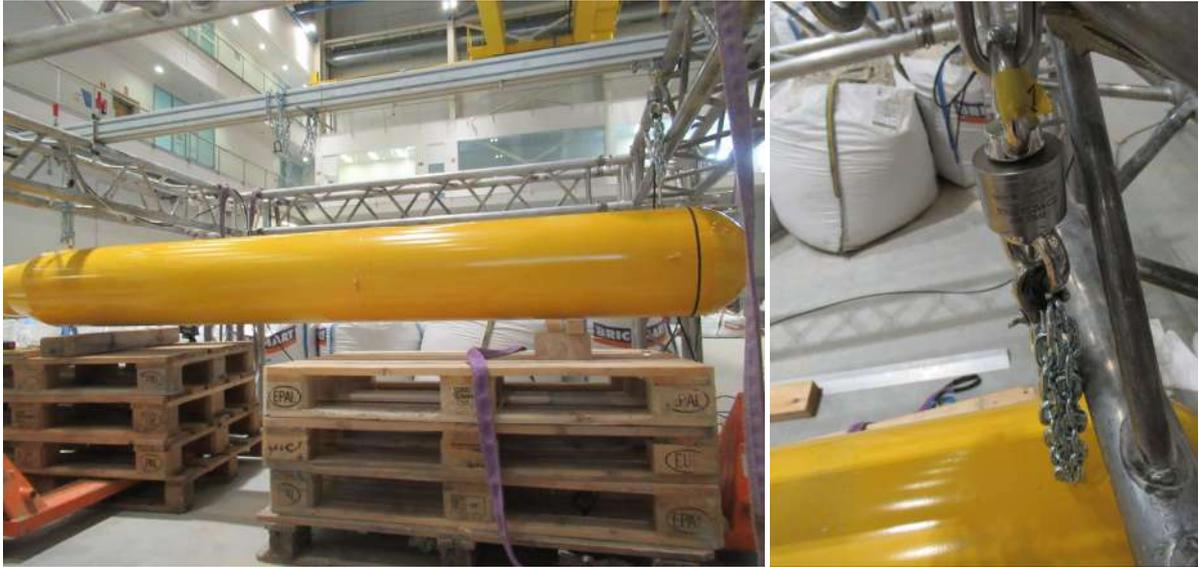
Figure 4-6. Weight and CoGz position test (left) and detail of hanging (right)
