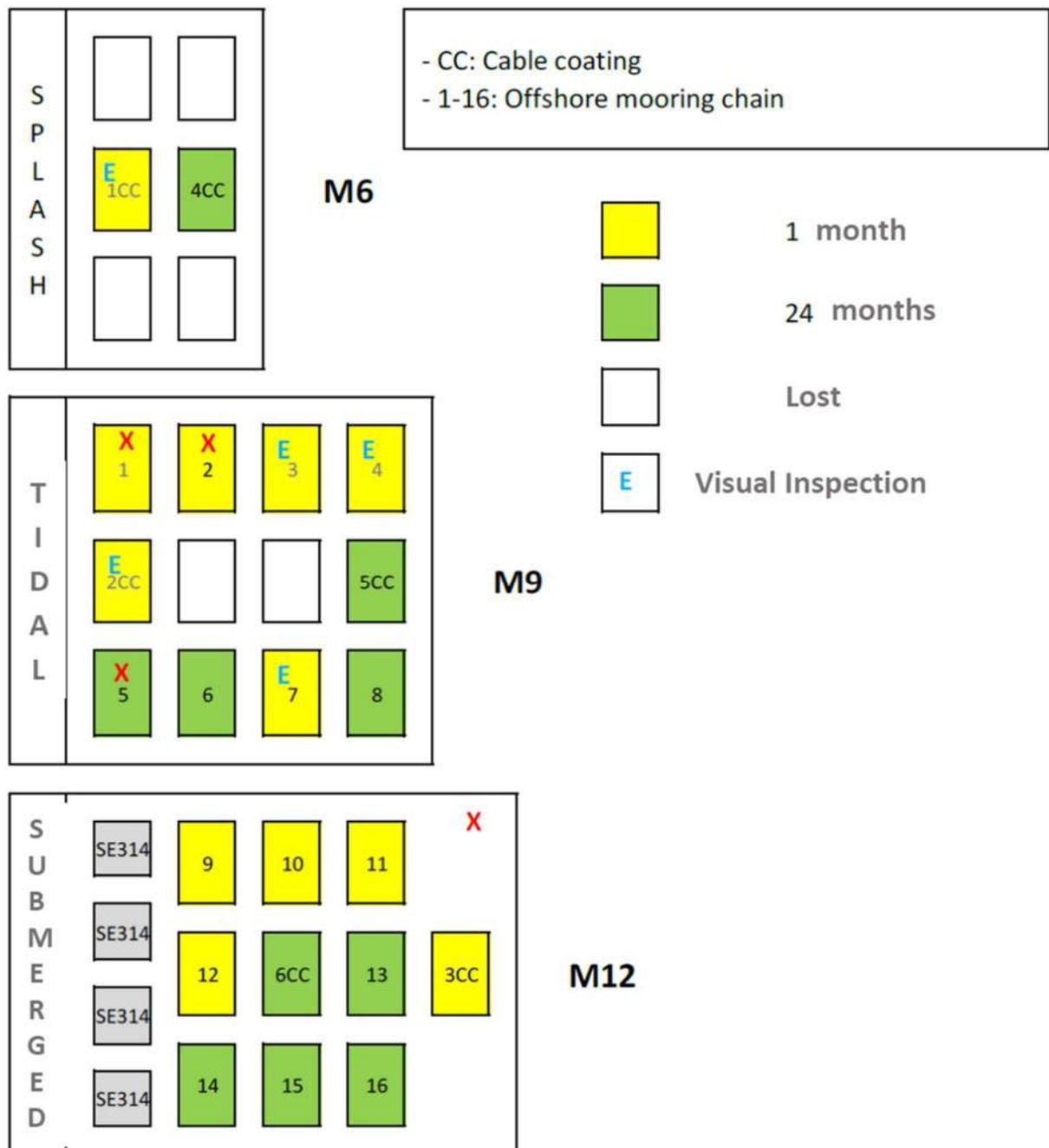
Figure 3-1. Schematic of the installed plates
