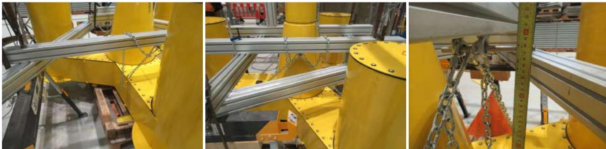
Figure 4-23.  $I_{xx}$  Inertia test (left)  $I_{yy}$  Inertia test (centre) and detail of hanging (right)
