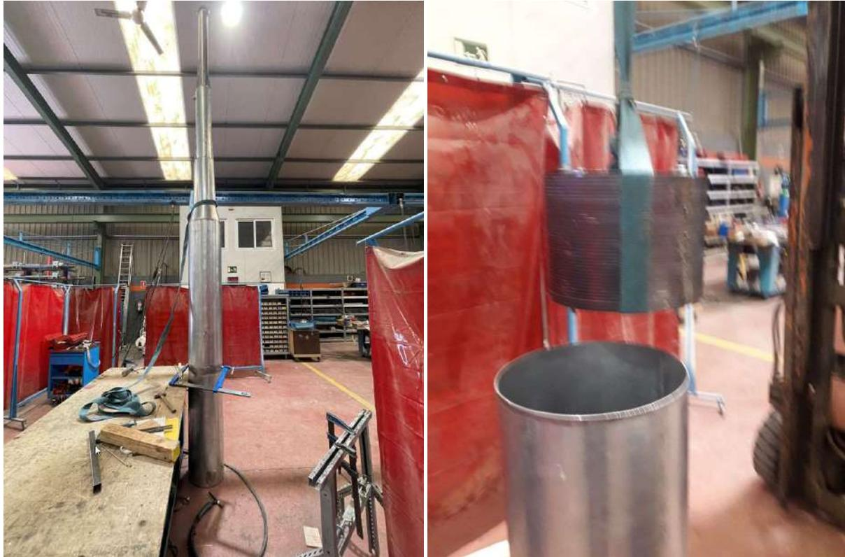
**Figure 4-4. WINDCRETE mockup being manufactured (left) with the ballast embedded (right)**
