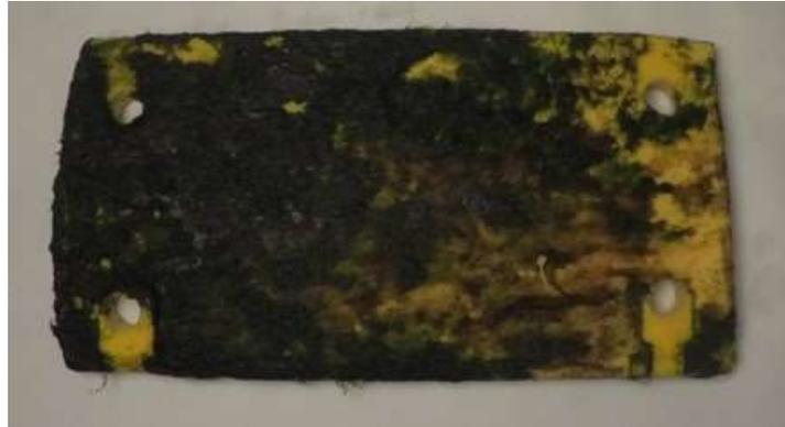
Figure 3-6. State of the cable coating plate extracted from the splash level.
