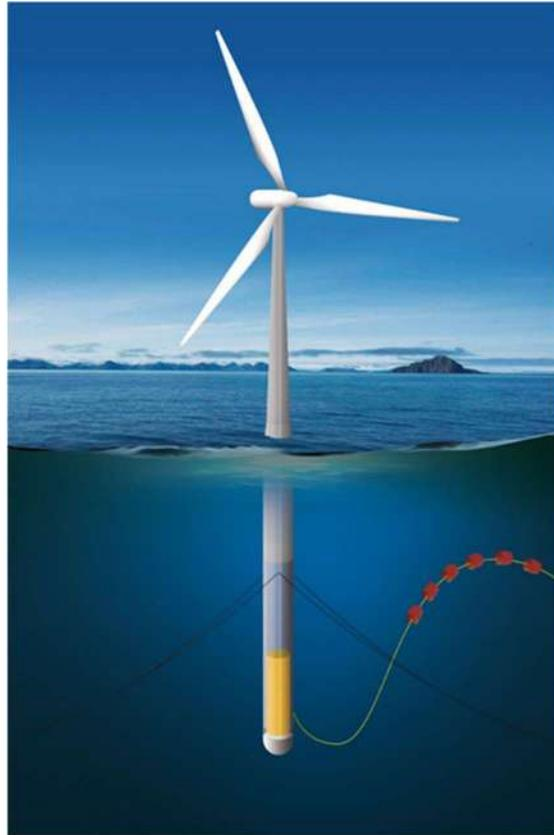
**Figure 3-1. WINDCRETE concrete-based concept of spar wind turbine**
