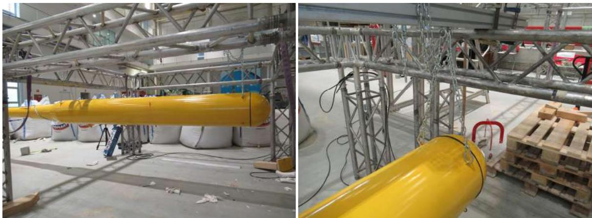
Figure 4-8.  $I_{zz}$  Inertia test (left) and detail of hanging (right)
