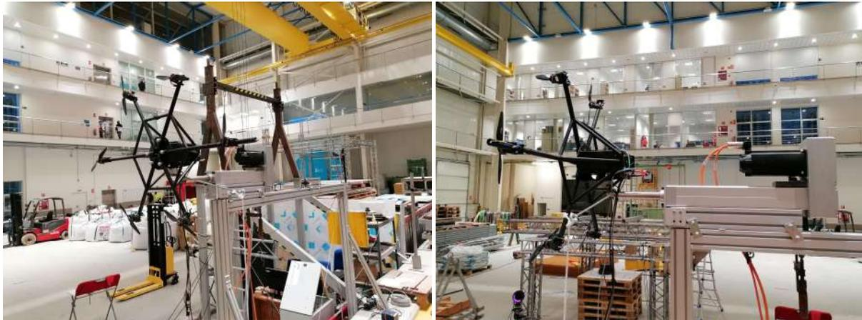
Figure 5-2. Setup of the FIHAC Multi-fan for the prescribed movements
