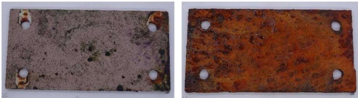
Figure 3-13. Plate # 6: Steel coated of Type 2 at Tidal area. Face A (left) and Face B (right)
