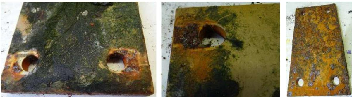
Figure 3-32. Plate # 3: detail of Face A (left), detail of Face A (centre) and Face B (right)
