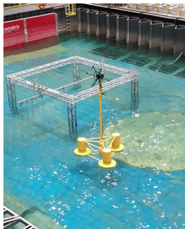
Figure 3-4. The multi-fan system at the Cantabria Coastal and Ocean Basin (Battistella, Meseguer, & Guanche, 2019).
