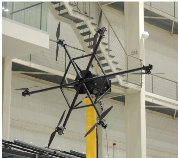
Figure 2-7. An overview of the multi-fan actuator system (Battistella, Meseguer, & Guanche, 2019).
