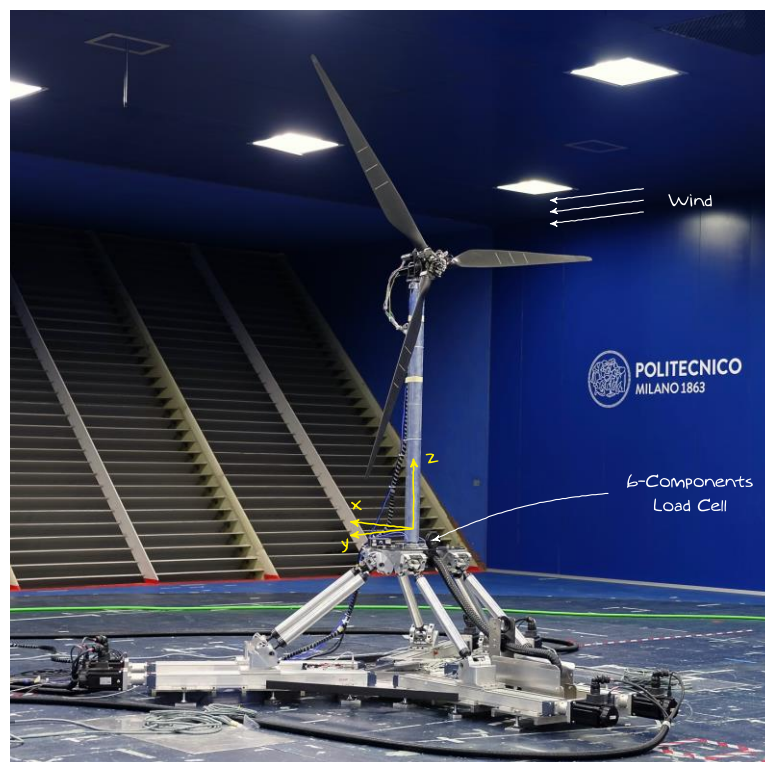
Figure 3-1. The hardware-in-the-loop system for wind tunnel hybrid experiments about floating offshore wind turbines.
