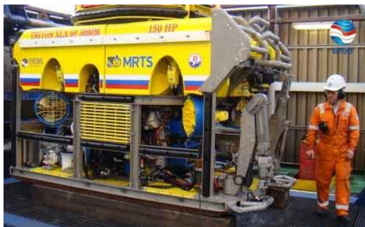
Figure 17: Class III ROV: XLX 150HP by Triton on a semi-submersible drilling rig, [source: [56]].
