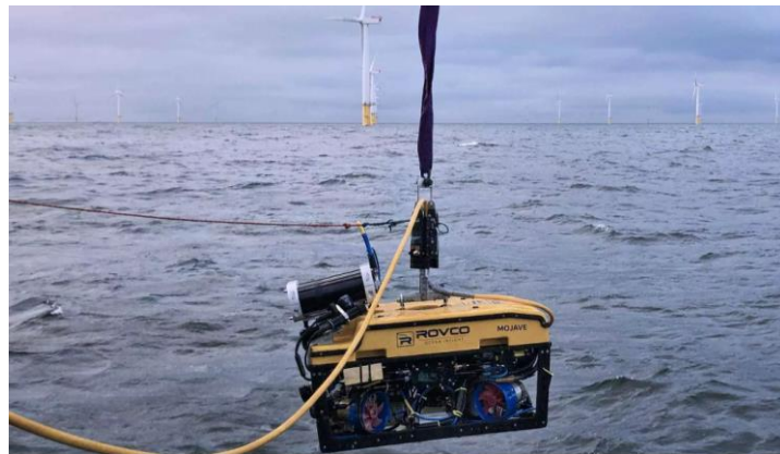
Figure 16: Mojave class II ROV by Rovco during free-swimming launch, [source: [54]].
