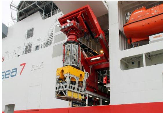
Figure 21: A-Frame preparing for launch, [source: [62]].
