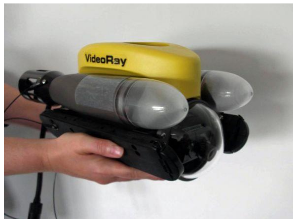
Figure 15: Class I ROV: VideoRay Pro 4 by VideoRay, [source: [53]].
