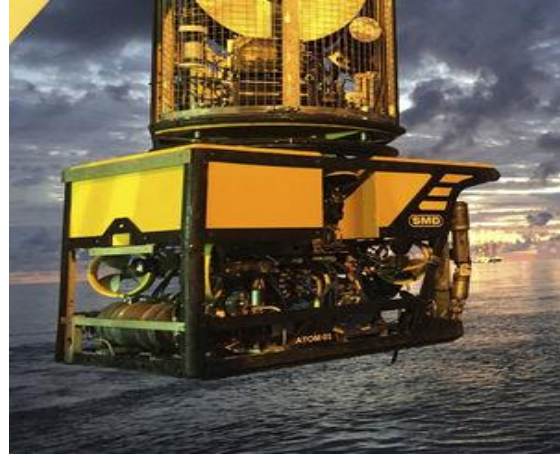
Figure 20: ROV being deployed with "top tat"-TMS, [source: [113]].
