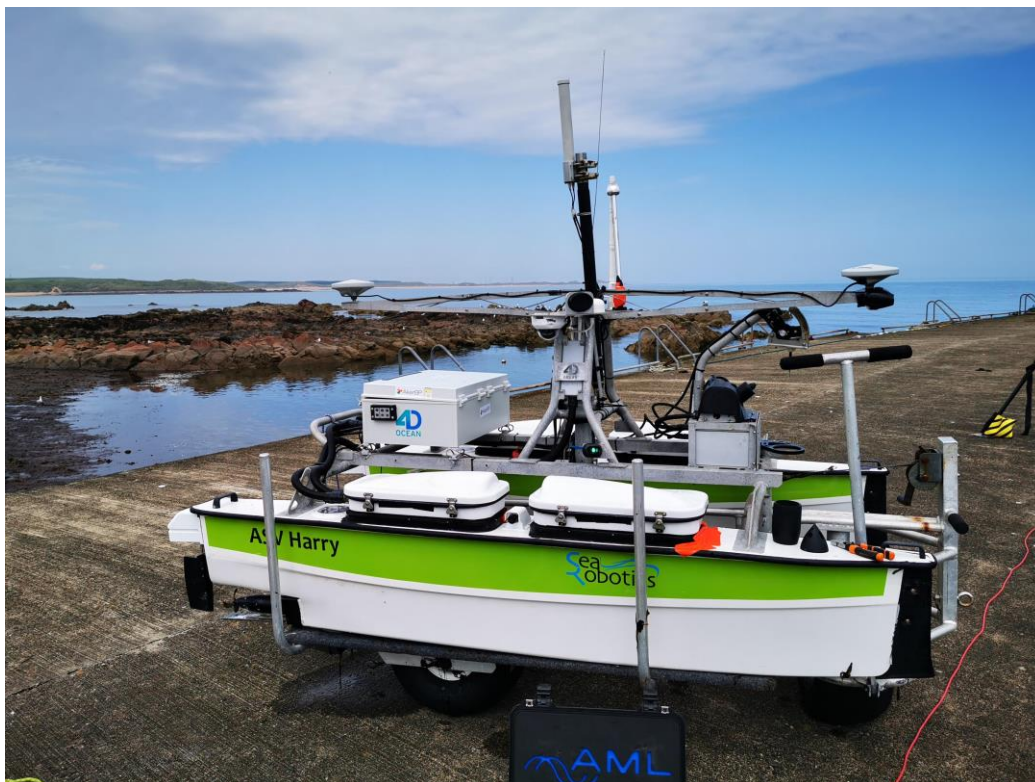
Figure 23: USV used to survey the export cable of Hywind Scotland Park, [source: courtesy of Equinor].
