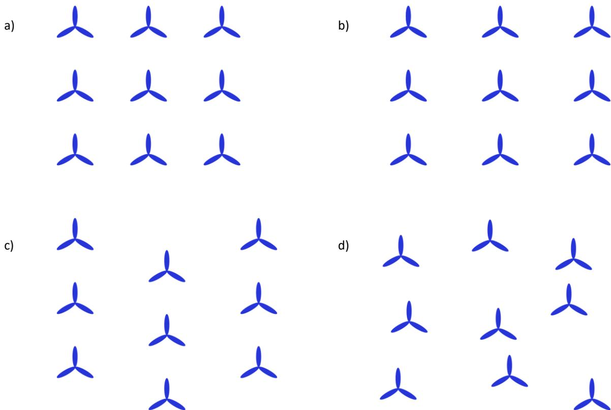
Figure 1. *Typical wind farm layouts: a) Rectangular matrix with equidistant turbines in both directions, b) Rectangular matrix with direction-dependent spacing, c) Staggered matrix and d) Irregular matrix.*
