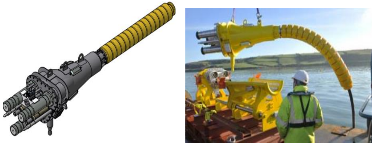
Figure 9.3-1 – MacArtneys 11kV Hybrid Wet Mate Connector Solution, Right: Male Connector, Left: Female and Male connector; Source: [31]
