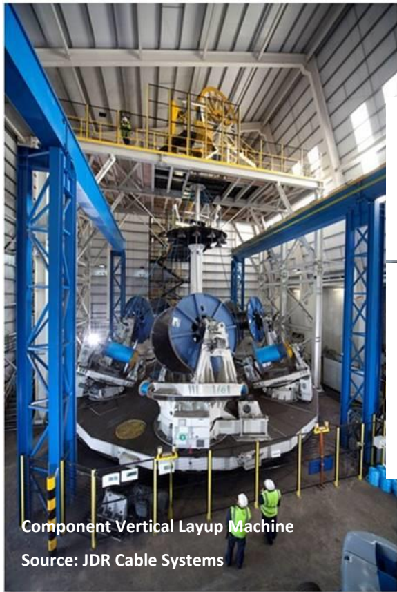
Figure 3.1-3 – Component layup operation and theory
