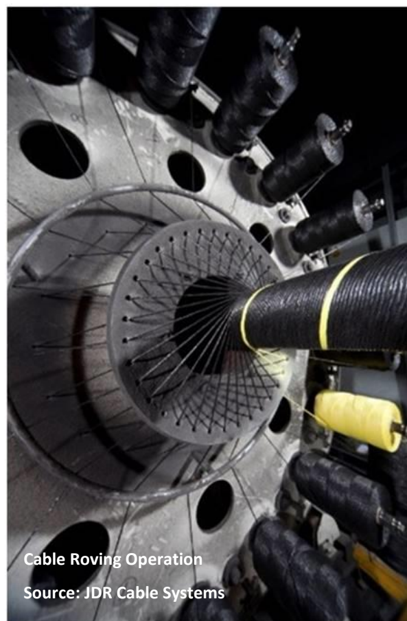
Figure 3.1-4 – Application of Armour Wire Reinforcement and Roving Layers illustrated
