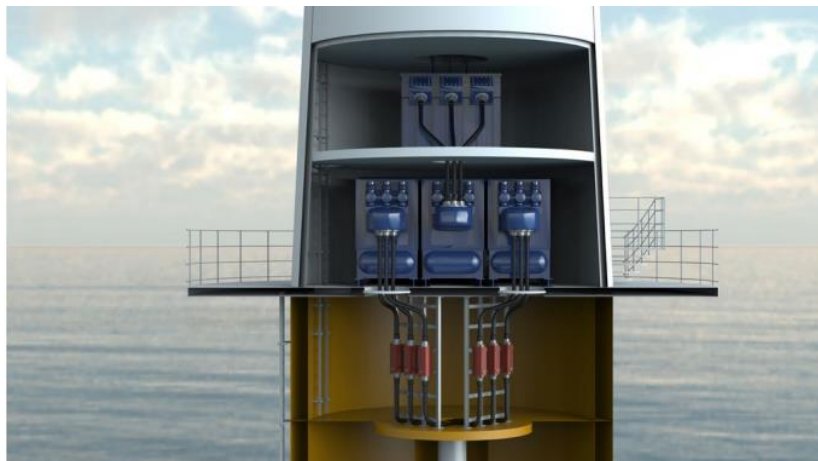
Figure 5.1-7 – Animation of a dry connection between sea and tower cable inside tower, Source: [14]
