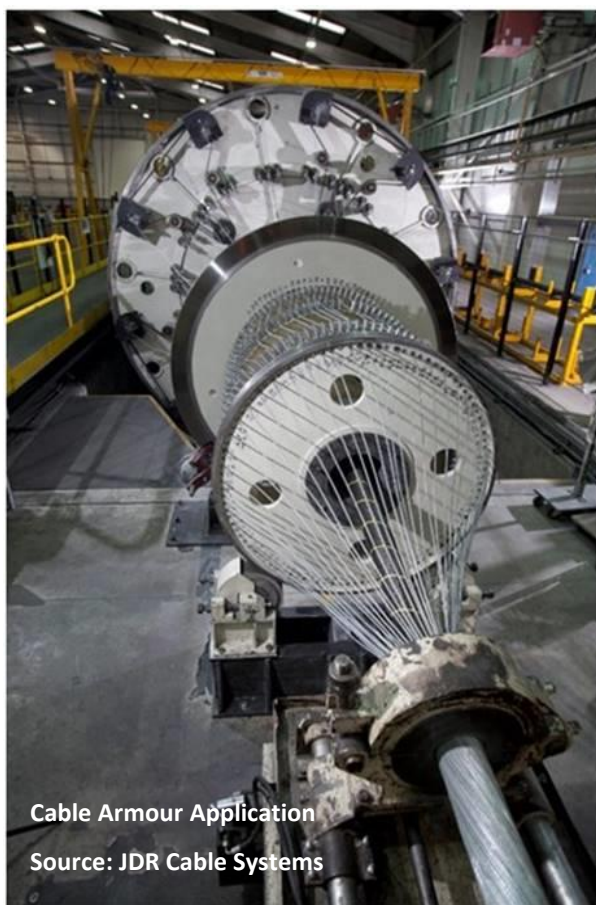
Figure 3.1-4 – Application of Armour Wire Reinforcement and Roving Layers illustrated
