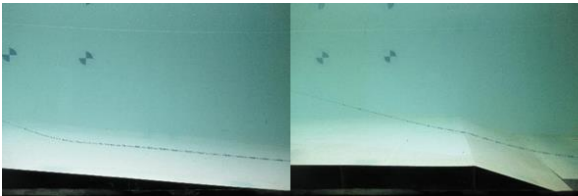
Figure 9- 1: Chain-nylon mooring configuration with gentle slope (left) and with steep slope (right) [17].
