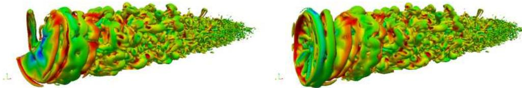
**FIGURE 27** Three-dimensional iso-vorticity contours over the last cycle of an extreme floater motion at 15 m/s. With an amplitude of  $6.38^\circ$  and a frequency of 0.11352 Hz. (Left) t2 and (right) t5 [Colour figure can be viewed at [wileyonlinelibrary.com](http://wileyonlinelibrary.com)]
