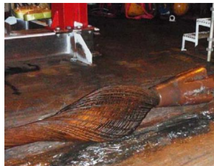
(b) Wire rope mooring line birdcaging due to compression near socket termination. Birdcaging can happen when the mooring line goes slack under large heave or pitch motions of the floating structure [Source: BP [15]].
