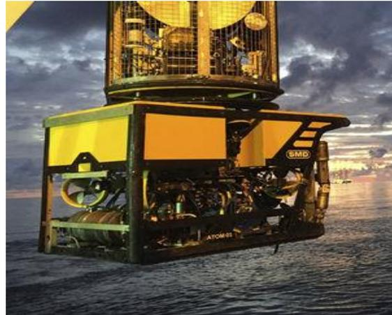
Figure 20: ROV being deployed with "top tat"-TMS, [source: [113]].
