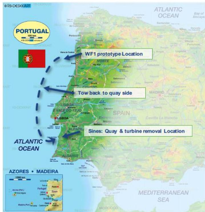
Figure 34: WindFloat1 prototype decommissioning map, [source: [101]].
