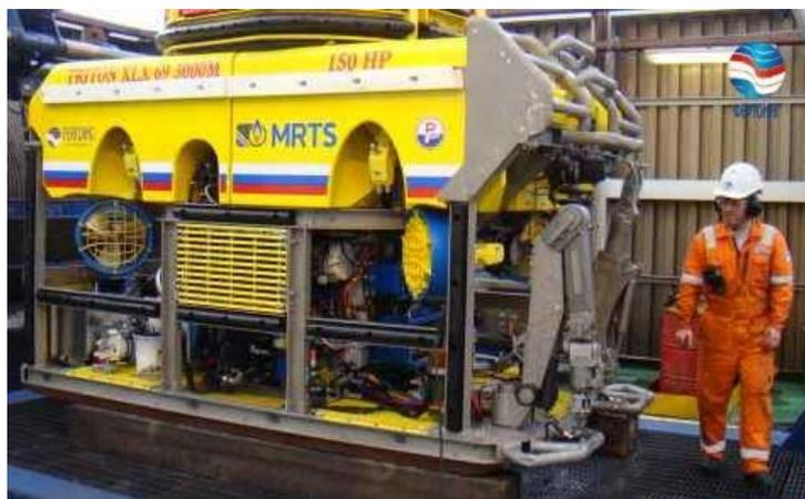
Figure 17: Class III ROV: XLX 150HP by Triton on a semi-submersible drilling rig, [source: [56]].
